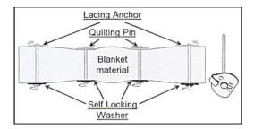
GEMCO lacing anchors and quilting pins are used in the manufacture of removeable blanket insulation.
